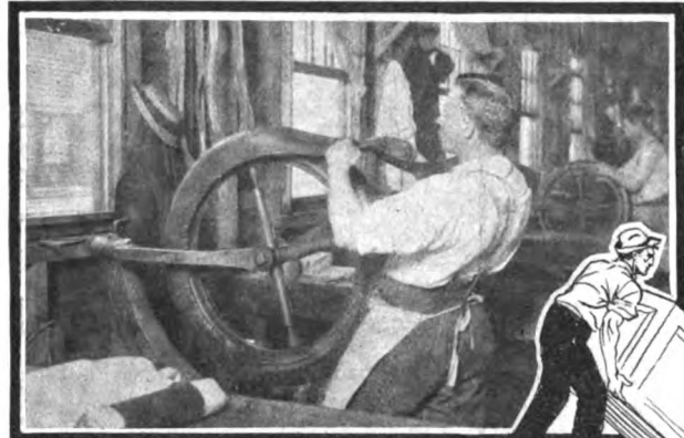
Stretching Fabric on Tire Form
